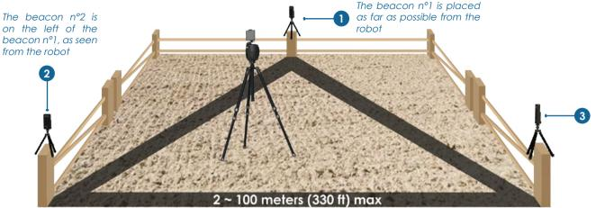
The positions of the beacons are very flexible, but tracking and accuracy are better with proper configurations:
