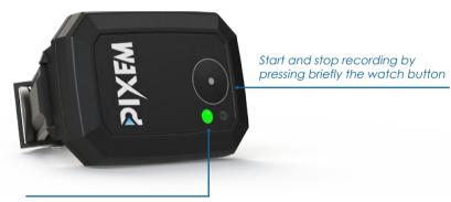
LED full green: recording command is ON LED blinking slowly: recording command is OFF
